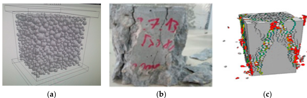
Figure 15. (a) Particle size distribution of the LDPM; (b) experimental crack pattern for the uniaxial test; and (c) crack pattern obtained by the LDPM simulation.
