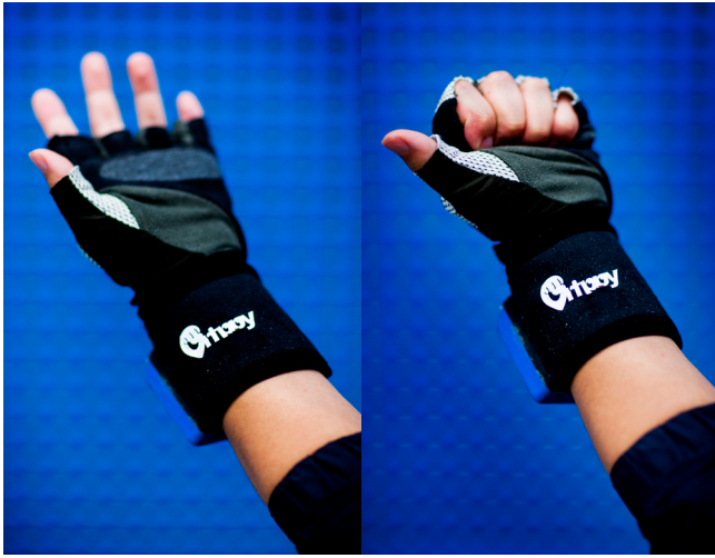
Figure 5.8. Intersecting with the haptic interface of Grippy (the glove-shaped version) by squeezing.
