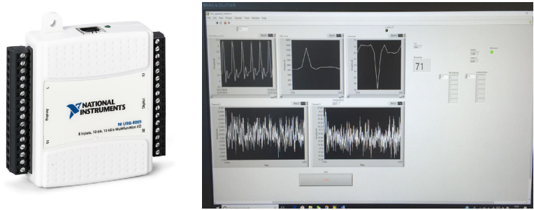
Figure 4.1. The device for data acquisition (DAQ 6009; left) and the interface of data processing software (LabVIEW; right).
