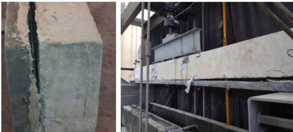
Fig. 24. Debonding at the interface [52,107].
