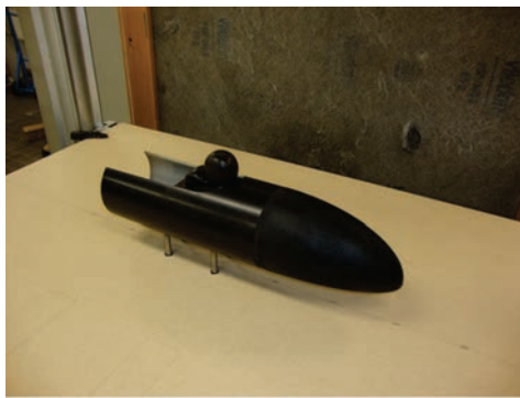
Fig. 5. (a) Simplified wind tunnel test set-up; (b) drag increase with nose rotation for Re = 1.58 \cdot 10^5 .
