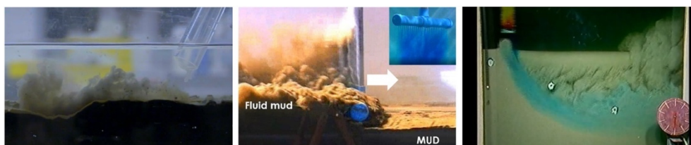
Fig. 8. Conducting laboratory experiments for understanding the physics of WID. A jet with a single nozzle (left and right panels) and with multiple nozzles (middle panel) are used for fluidizing consolidated mud and creating a density current.
