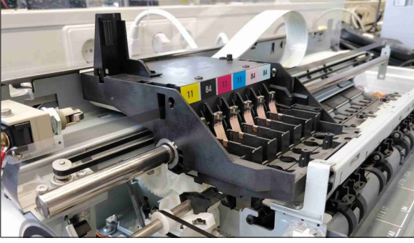
Fig. 4. Printer motion system with: motor, drive belt, slide guide, and carriage with printhead
