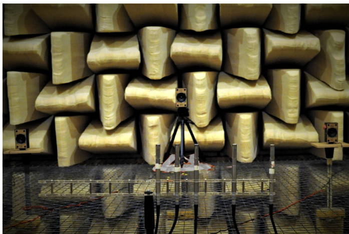
Figure 4.10: Picture of the experimental setup considering five AVSs and three speakers, located at a radius of r = 3.6 m.
