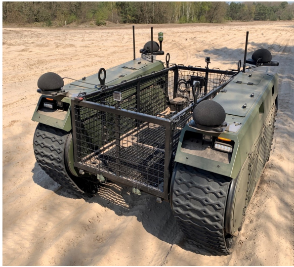
Figure 1.4: The outdoor version of the AVS array deployed on a vehicle [5].
