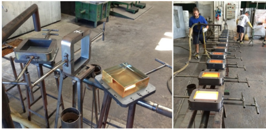
Fig. 6. High precision open steel moulds used for the manufacturing of the glass blocks for the Crystal Houses project.
