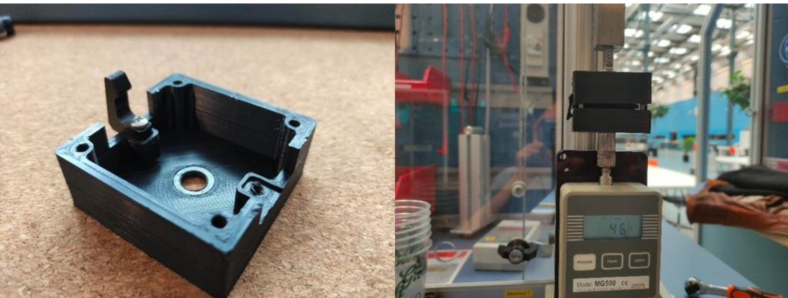
Figure 31 - (left) Jig and (right) force gauge with jig installed to measure tensile and compression forces on snap fits. Used with approval of M. Bakker, 2021.
