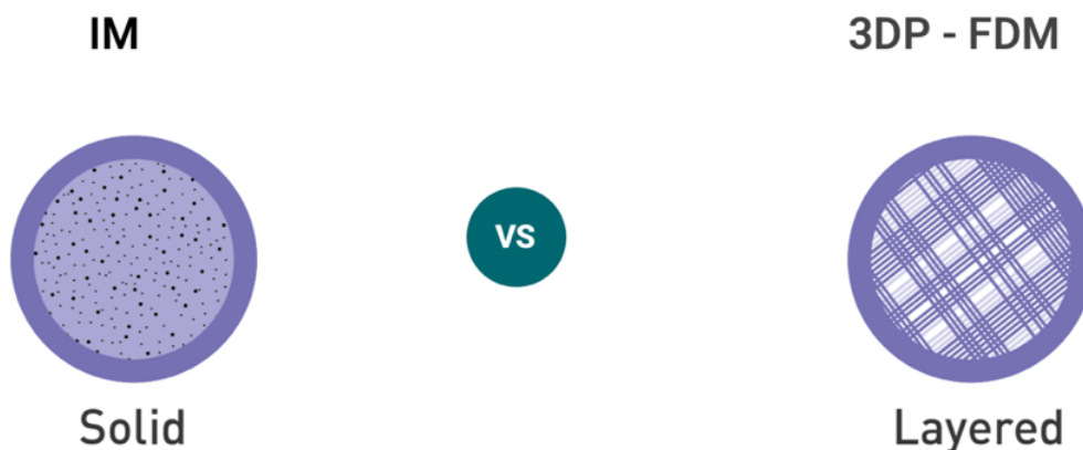
Figure 13 - Internal Structure of IM parts and FDM parts.
