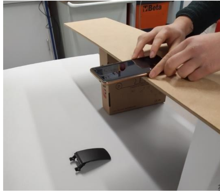
Figure 22 - Set up to take pictures as perpendicular to the object as possible.
