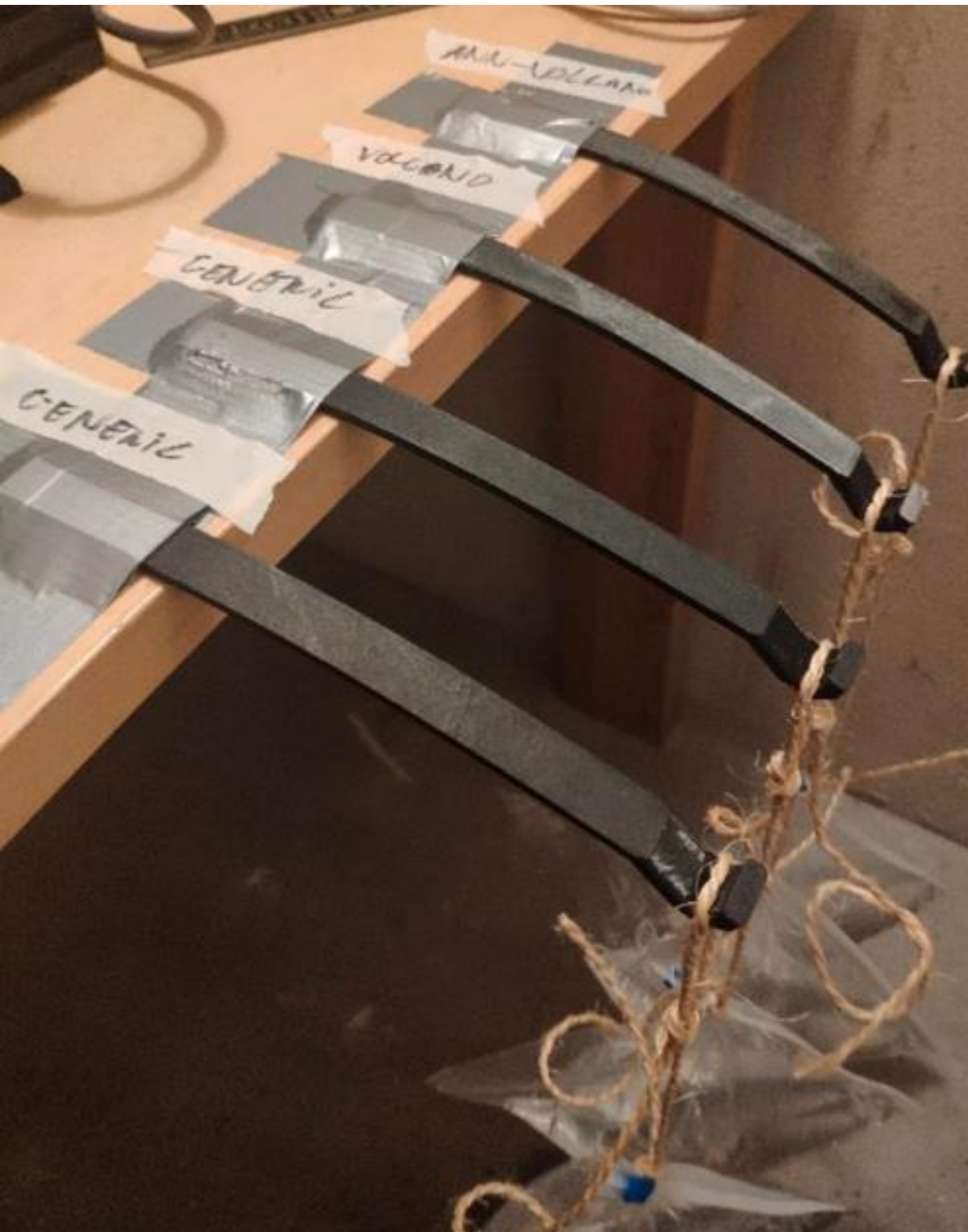
Figure 32 - Home-made creep test, used with approval of N. Van Silfhout, 2020.
