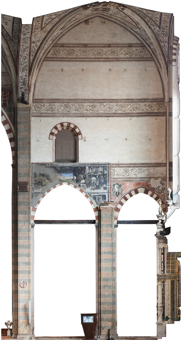
Fig. 3. Section of the transept towards the Pisanello's fresco, photogrammetric reconstruction (G. Verdiani, 2021).
