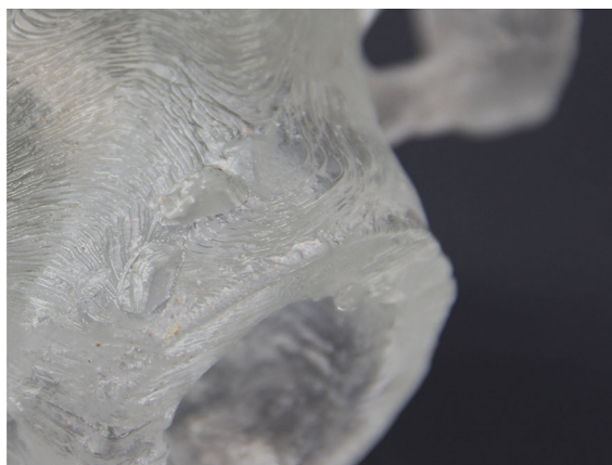
Fig. 30 Rough surface of lost-wax cast element showing traces of the FDM printing
