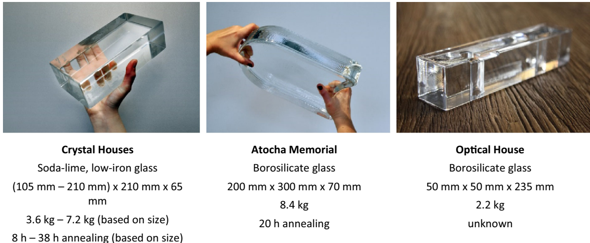
Fig. 2 Characteristics of the solid glass brick units of some of the most representative envelopes made of solid glass components. Derived from (Oikonomopoulou 2019). Right and center photo image credits: F. Oikonomopoulou. Left image credits: Hiroshi Nakamura & NAP
