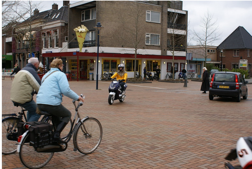
Figure 3. 'Shared space' design of a road crossing where there is no clear demarcation between areas for pedestrians, cyclists and cars—as well as no signs and traffic lights, thereby tapping into road users own responsibility to look out for others (source: Fietsberaad, CC BY-ND 2.0)
