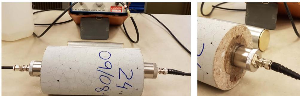
**Fig. 2.** Direct UPV measurements.
