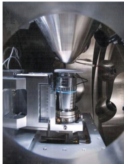
FIG. 3. (Color) View of integrated optical microscope in SEM chamber.
