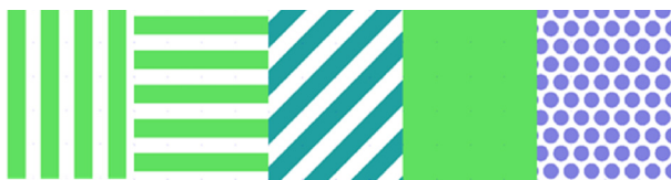
Fig. 6. (Color online) Calibration sample: the color part is electron transparent area and the white is tungsten. Lines: 0.5\text{ }\mu\text{m} wide, 1\text{ }\mu\text{m} pitch; holes: 0.4\text{ }\mu\text{m} diameter, 0.6\text{ }\mu\text{m} pitch.
