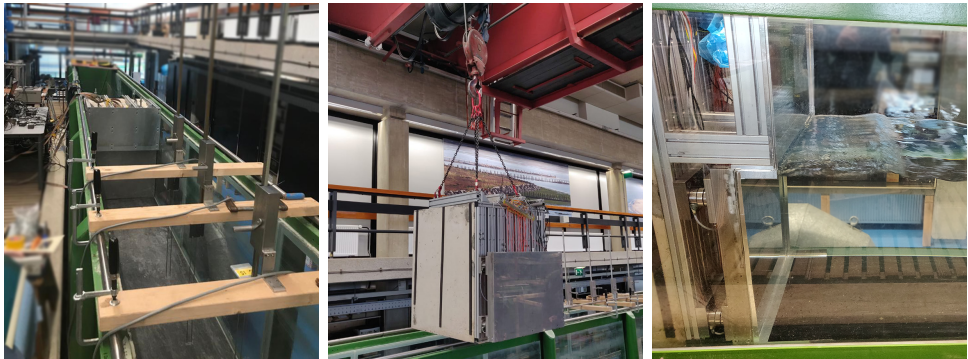
Figure 5.2: Impressions of the experimental facility and setup. The concrete block is placed in the wave flume. On the photo on the right, the front steel plate of the overhang and tapes on the sides of the gate to ensure water tightness have not yet been installed.
