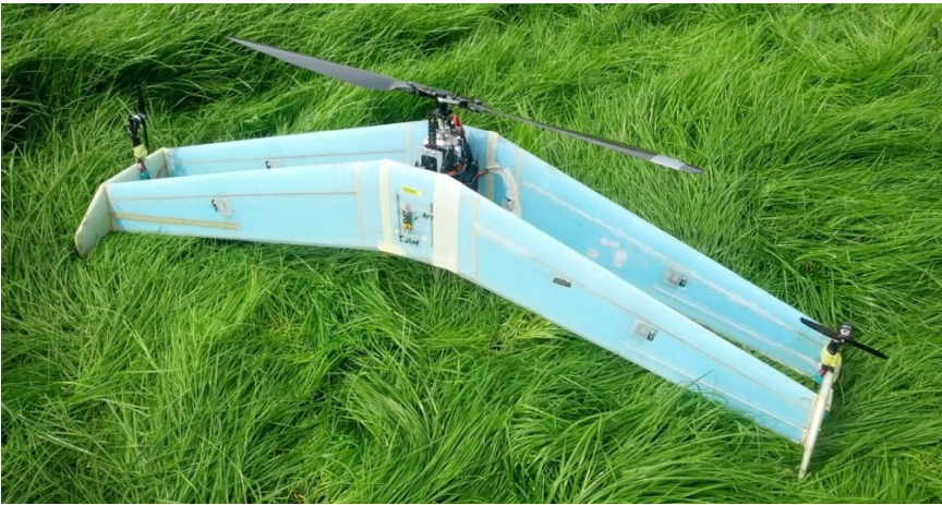
Figure 5.1: Novel hybrid Unmanned Air Vehicle featuring a cyclic and collective pitch controlled rotor combined with a biplane deltawing.
