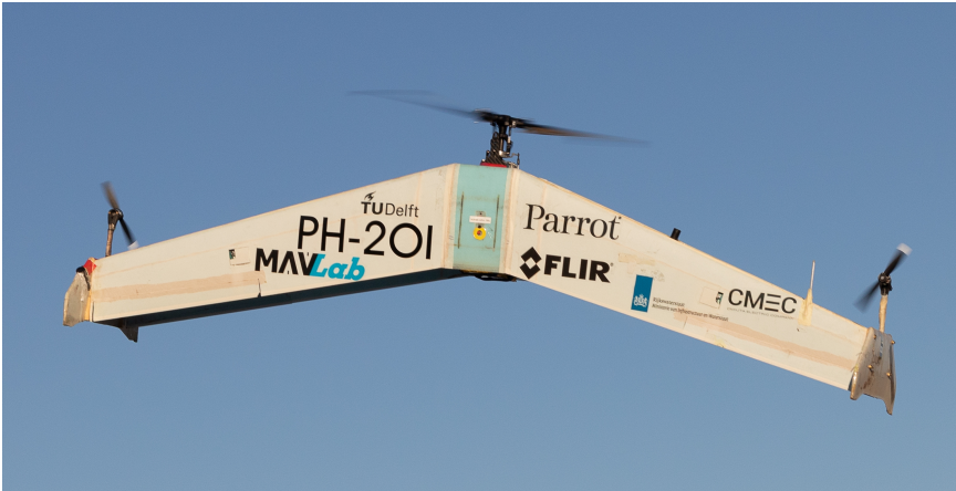
Figure 7.1: The DelftaCopter tailsitter UAV in hovering flight. DelftaCopter has a single large rotor with collective and cyclic blade pitch control, two small torque countering tip propellers, and a pair of delta-wings placed in a biplane configuration. The tips form the landing legs and provide yaw stability in forward flight. It weighs 4.3 kg and was designed to fly 60 km in the Outback Medical Challenge 2016 [6] [7]
