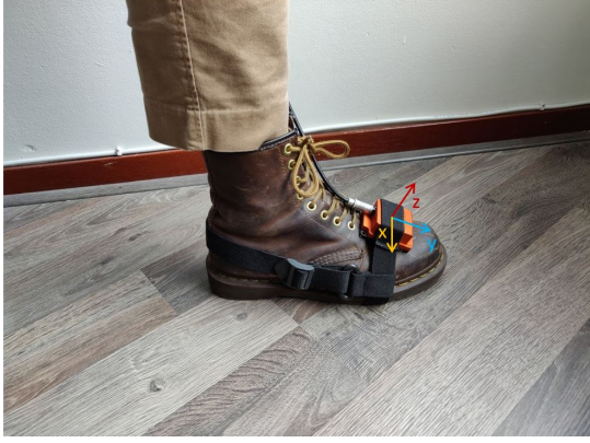
Fig. 2. Experimental setup with foot-mounted sensor.
