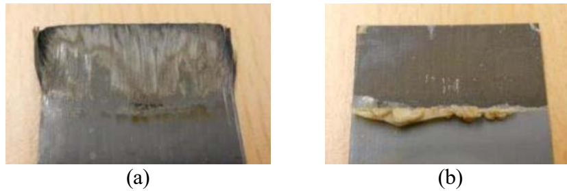
Figure 6: Representative CF/epoxy fracture surfaces after (a) direct welding under long-heating-time conditions, and (b) indirect welding under short-heating-time conditions. (Adapted from [13].)
