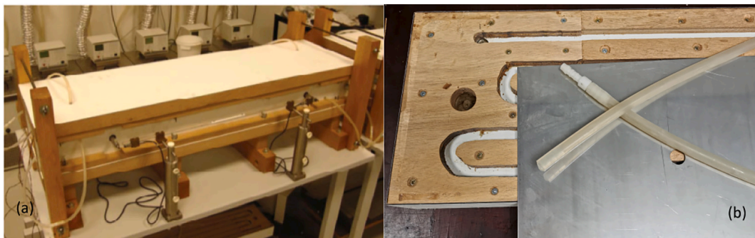
Fig. 2. (a) An ADTM used for deformation measurement. (b) Configuration of the mould, made by foam, wood, rubber tube and steel plate. Canals were cut in the inner surface of the mould.
