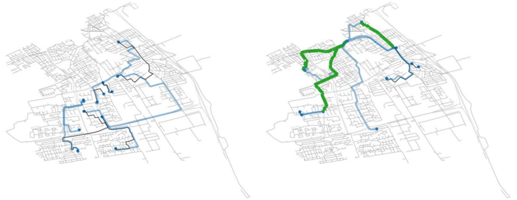
Fig 8. Traces of rides for a single simulated vehicle without (left) and with pooled ride services (right). Blue—single traveller on-board, Green—several travellers sharing a ride, Black—empty vehicle trip.
