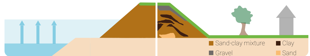
A homogeneous vs a variable dike interior providing flood safety under increasing river water levels. Based on schemes from Teun van Woerkom.
