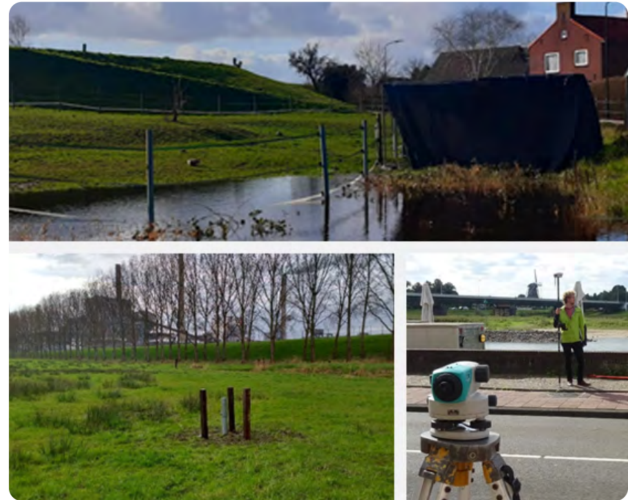
Figure 2: Top: Seepage through the dike and the subsoil (Photo by Waterschap Rivierenland). Bottom: Tube that is placed in the soil to measure the groundwater (Photo by Waterschap Brabantse Delta) and fieldwork for data collection (Photo by Bas van der Meulen).
