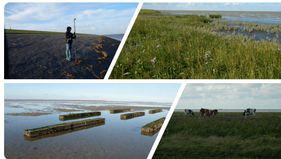
Figure 2: Top-left: measurement of beach wrack on the dikes after a storm, as a measure for wave run-up. Top-right: salt marsh edge. Bottom-left: biodegradable artificial reefs deployed in the tidal flats of Griend. Bottom-right: cattle grazing in a salt marsh. Photos by Beatriz Marin-Diaz.
