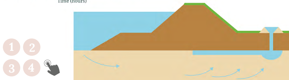
The development of the pipe length during a high water event. Based on schemes by Joost Pol.
