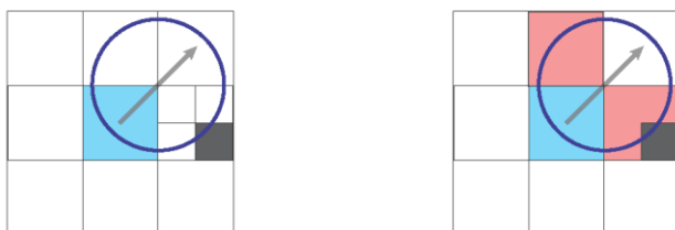
Figure 10: Collision avoidance: The area that must be checked for occupied nodes
