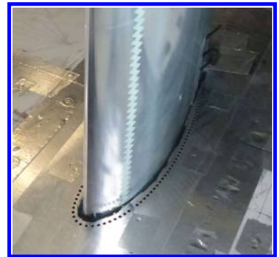
Fig. 5 Holes in the side plate around the main element of the wing for the suction system.
