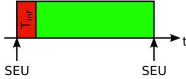
Figure 5.6: Fraction of time where inferences are wrong (red) because of SEUs (case without EDAC). A similar figure holds when parity is employed, where the red is replaced by yellow (unavailable). Fraction of times are not to scale.
