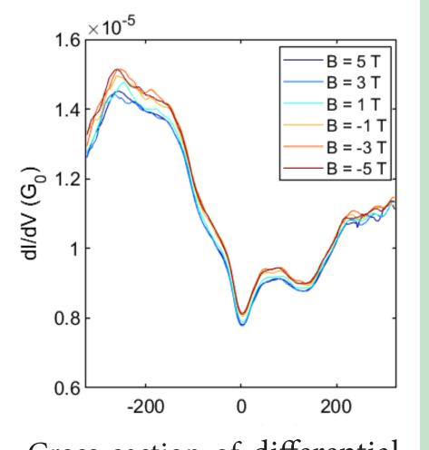
Cross section of differential conductance in magnetic field sweep: The dip position is independent of the magnetic field applied.
