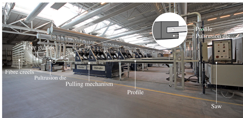
Fig. 2. A state-of-the-art, industrial resin-injection pultrusion line. Here, the material flows from left to right (courtesy of Fiberline Composites A/S). A schematic of the line can be seen in Fig. 3 and a cut-view schematic of the pultrusion die can be seen in Fig. 4. This figure was taken from Sandberg [10].
