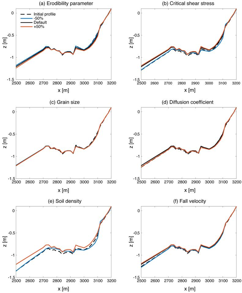
Figure C.2: Sensitivity analysis of the results for a 2-day storm period with  $H_s = 2$  m and  $T_m = 7$  s with respect to (a) the erodibility parameter  $m_e$ , (b) the critical shear strength  $\tau_{cr}$ , (c) the mean grain size  $D_{n50}$ , (d) the diffusion coefficient  $D$ , (e) the soil density  $\rho_s$ , (f) and the fall velocity  $w_s$ .
