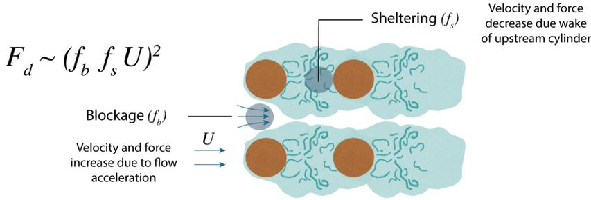
Figure 6.1: Parameterization of the drag forces acting on a cylinder in a current. The velocity upstream of the cylinders is multiplied by a blockage factor ( $f_b$ ), which accounts for flow acceleration between cylinders, and by a sheltering factor ( $f_s$ ), which accounts for the velocity reduction on downstream cylinders due to wake development.
