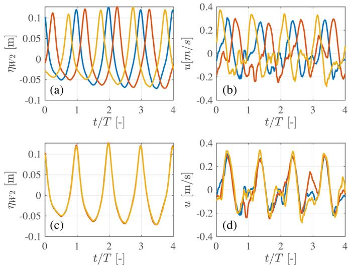
Figure B.2: The upper plots show the surface elevation (a) and the flow velocities (b) at tests where the velocity measurements were collected at different heights from the bed for  $1C$  and  $T = 3$  s, prior to shifting the time series. The lower plots show the surface elevation (c) and velocity (d) measurements after time shifting the time series.
