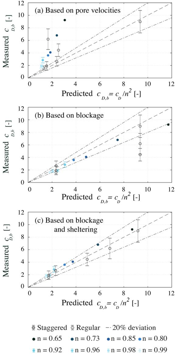
Figure 2.4: Predictions versus bulk drag coefficient ( $c_{D,b}$ ) measurements for random cylinder arrays, by Tinoco and Cowen<sup>150</sup> and Tanino and Nepf<sup>146</sup>, and versus measurements for regular and staggered arrangements by Jansen<sup>68</sup>. Plot (a) shows  $c_{D,b}$  values calculated from the pore velocities, (b) from the blockage factor and (c) from the present model. Vertical bars show the estimated measurement error.
