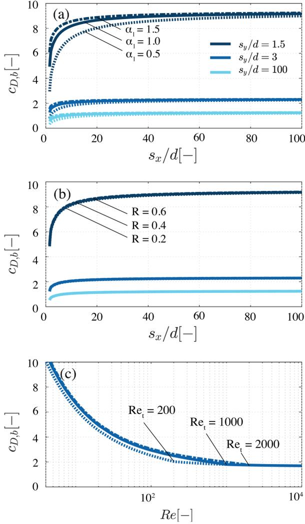
Figure 2.6: Sensitivity of the modelled bulk drag coefficient  $c_{D,b}$  to varying values of (a) the scale factor  $\alpha_1$  and (b) the correlation factor  $R$ , as a function of the streamwise spacing  $s_x$  and spanwise spacing  $s_y$  between cylinders compared to the cylinder diameter,  $d$ . Plot (c) shows the influence of the limit for turbulent flow,  $Re_t$ , on the bulk drag predictions for  $s_y/d = 1.5$  as a function of the Reynolds number  $Re$ .
