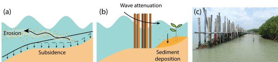
Figure 4.2: (a) Increase of the water level at the coast due to subsidence and erosion. (b) Foreshore restoration using permeable structures, which attenuate waves and enhance deposition landwards from them. Since the structures only restore the area behind them, in order to continue expanding the shoreline, a new structure should be built offshore from the old one in posterior stage. (c) Photograph of a bamboo and brushwood structure in Demak, Indonesia.
