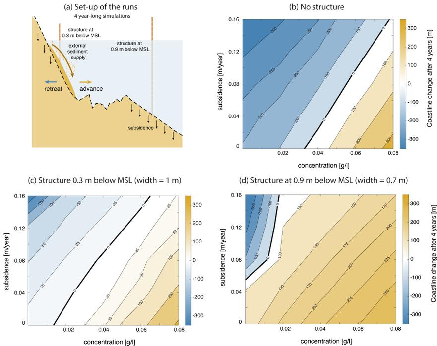
Figure 4.11: Evolution of the coastline of Demak over 4 years for several scenarios of subsidence and external sediment supply, such as rivers. The set-up of the runs is shown in plot (a). The results are presented for a situation without structures (b), with a structure placed at 0.3 m below MSL (c), and with a structure placed 0.9 m below MSL (d).
