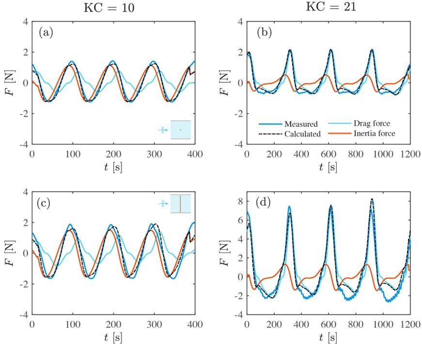
Figure 3.8: Comparison between measured and fitted forces for  $KC = 10$ , and configurations (a) 1C and (c) D, and for  $KC = 21$ , and configurations (b) 1C and (d) D. The measured force signal is shown in black, and the fitted signal in dark blue. The fitted force is decomposed in the inertia component (red) and the drag component (blue). For lowest  $KC = 10$  (a,c) the force signal is dominated by inertia, whereas for  $KC = 21$  (b,d) it is driven by the drag component.
