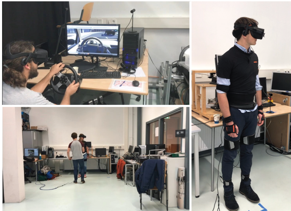
Figure 1: Driver (left top), pedestrian during a trial with an experimenter monitoring safety (left bottom), and pedestrian with motion suit (right).
