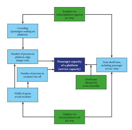
Figure 3.8: Relationships between the limits on the passenger capacity of a platform
