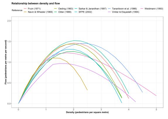
Figure 3.7: Fundamental diagram for pedestrian traffic (flow-density relation)
