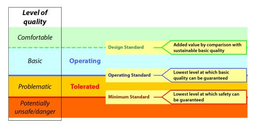
Figure 3.5: Definitions of Minimum Standard, Operating Standard and Design Standard (from [77])
