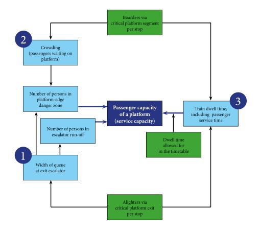
Figure 1: Relationships between the limits on the passenger capacity of a platform
