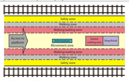
Figure 3.6: Functional characteristics taken into account when determining platform width (from [78])
