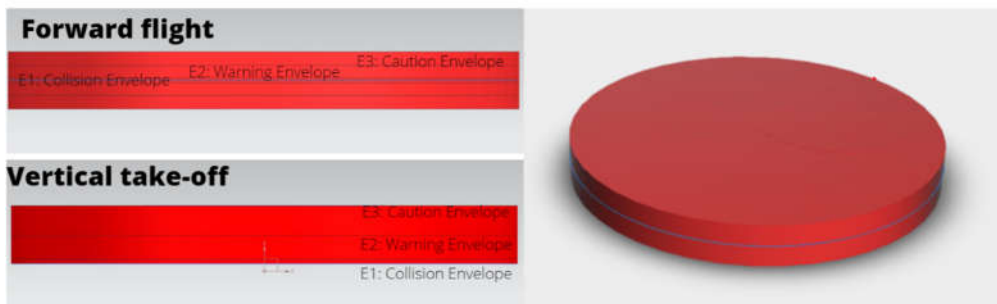
Figure 4: On the left side, in the top half, the layers of the safety envelope in forward flight are shown from a side view. In the bottom half, the layers of the safety envelope in vertical flight are shown from a side view. On the right side, the general setup of the entire safety envelope in three dimensions is shown.
