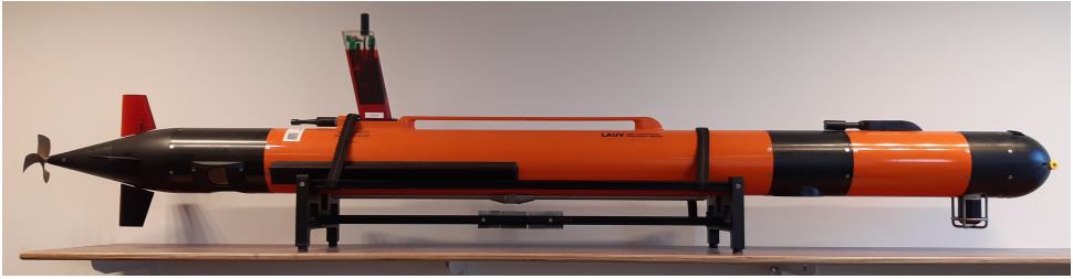
Figure 1.3.: Lightweight Autonomous Underwater Vehicle of OceanScan-MST.
