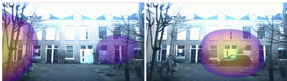
(c) sound localization with a vehicle-mounted microphone array detects the wall reflection of an approaching vehicle behind a corner before it appears
