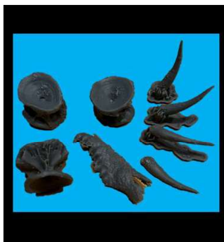
Figure 6.8 Examples of 3D prints of fish bones. S3-26 pike vertebra seen from a different point of view, S3-13 jaw and S3-2 pike tooth on a display stand. Magnification \times 10 . The pike tooth replica is 5.5 mm long.
