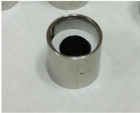
3 FIGURE 4 a. Sample in Storage Container, Showing the Silicon Paper That Controls Contact Area d. 4 Assembled Test Specimen with Weight.
