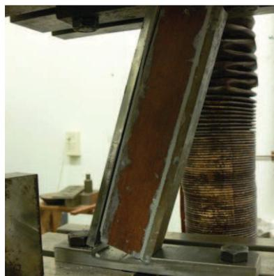
**Figure 10:** Massaranduba specimen: Failure of 100% in the glueline.
