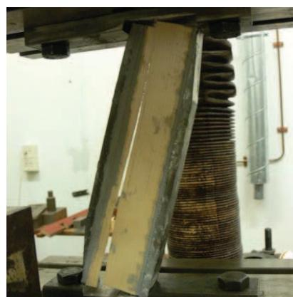
**Figure 12:** Spruce specimen: Failure of 0% in the glueline.
