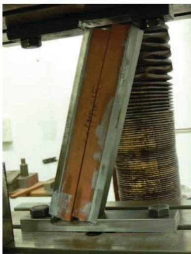
**Figure 11:** Massaranduba specimen: Failure of 0% in the glueline.
