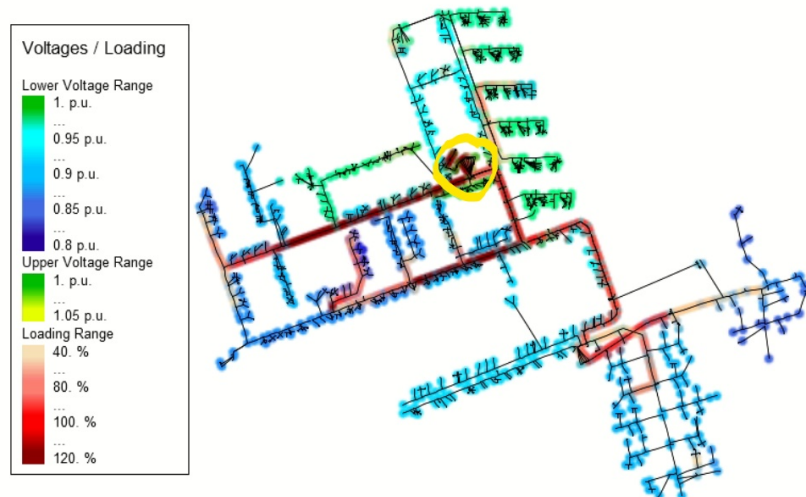
Figure 10. Grid loading heatmap of SUB1 grid with PSM with EV 80% penetration in winter, highest line loading moment.
