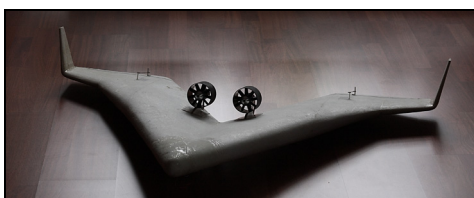
FIGURE 27. With the engines and batteries the weight of the model was increased to 1400g. The required speed for the design C L is then 50km/h. As engines electro impellers were taken. The batteries were installed in the underbelly.
