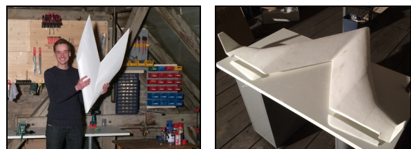
FIGURE 23. The wings were glued together with styrofoam glue and smoothed with sand paper. The flaps were cut out and the model was covered in a thin layer of glass fiber.
