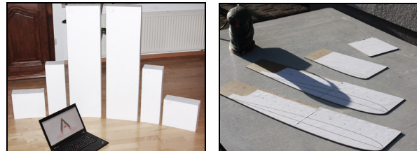
FIGURE 21. Blocks for the wing elements were cut with a hot wire cutter and the profiles were cut out of wood
