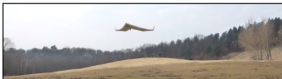
FIGURE 26. First flight of the Flying V (28.02.2014, Berlin, Germany): The model was thrown from a little hill out of a height of roughly 3.5m. After a short and fast descent to gain speed after the throw a straight glide path could be taken up on which the Flying V flew roughly 90m. The airplane was easy to control and landed smoothly.
