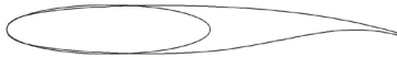
FIGURE 4. Efficient use of space with a cylindrical pressurized section which cuts through the plane of the airfoil in the shape of an ellipse
