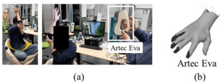
Figure 2: 3D scanning of human hands using Artec® Eva® scanner, courtesy of [9]
