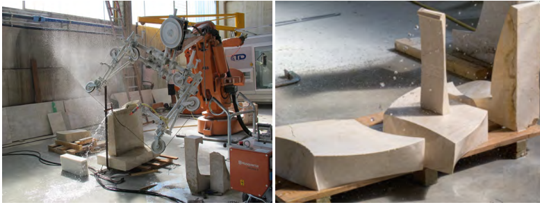
Figure 3.5: Robotic abrasive wire-saw cutting of marble blocks at Carrara, Italy (left); cut samples (right)
