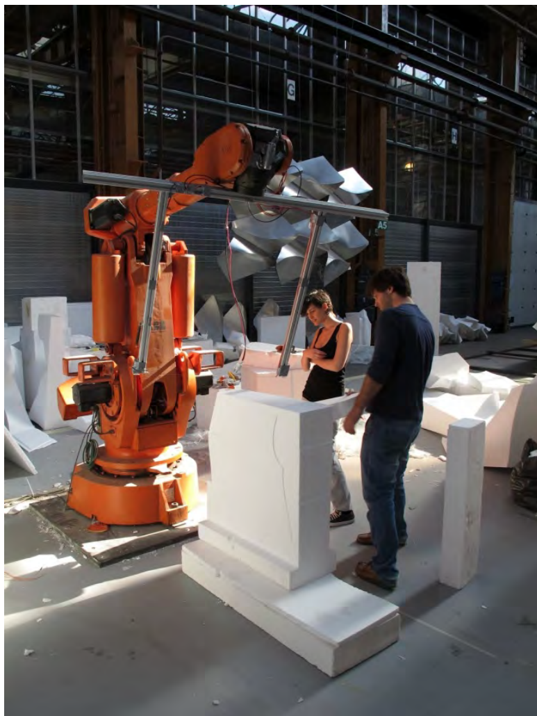
Figure 2.26: Production of the RDM Vault at Hyperbody's robotics workshop in Rotterdam
