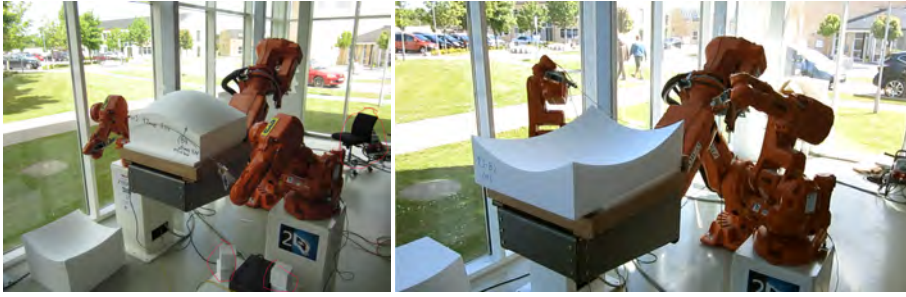
Figure 3.15: Tri-robot hot-blade cutting configuration
