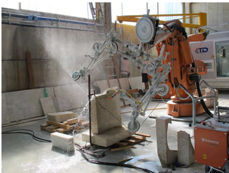
Figure 2.45: Diamond sawing of excess marble
