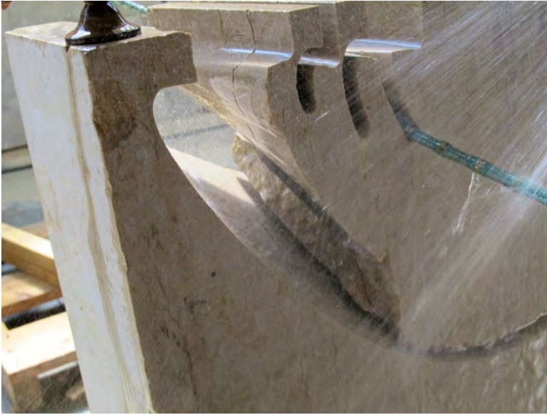
Figure 2.44: Experimental diamond wire saw setup
