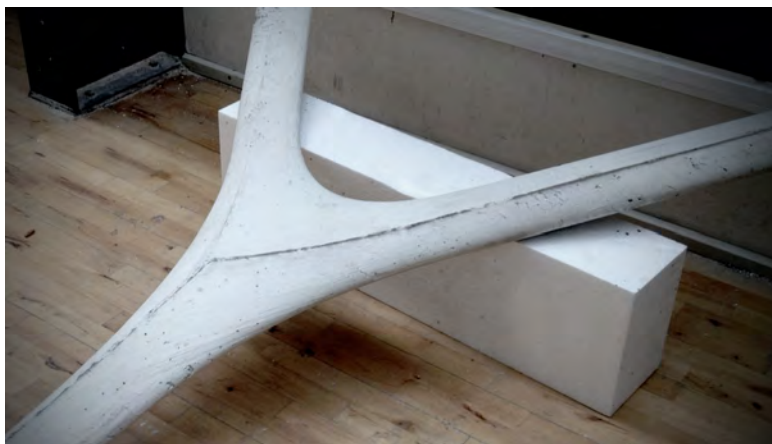
Figure 2.50: Y-joint sample cast constructed from three intersecting hyperboloidal surfaces and six single-ruled extrusions
