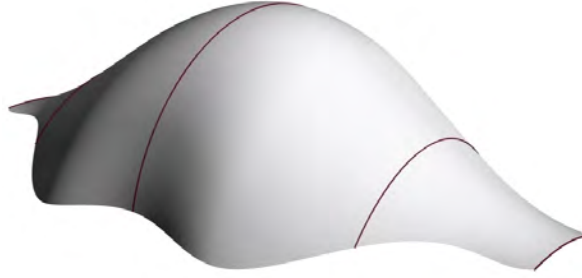
Figure 3.9: Elastica surfaces generated through implementation of the above formulation in Matlab
