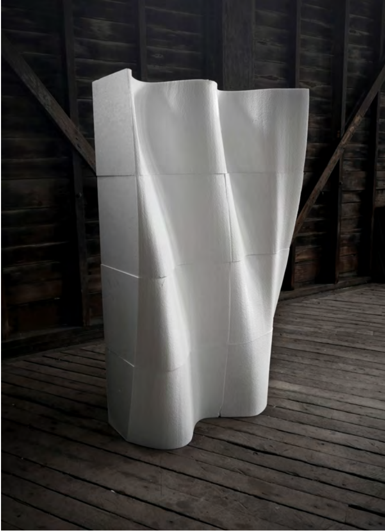
Figure 4.7: Early doubly-curved hot-blade demonstrator produced at the Robarch 2016 Workshop, “SuperForm”, by the BladeRunner Research consortium and workshop participants
