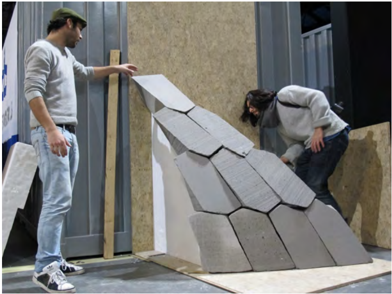
Figure 2.43: Initial test cuts in engineered limestone
