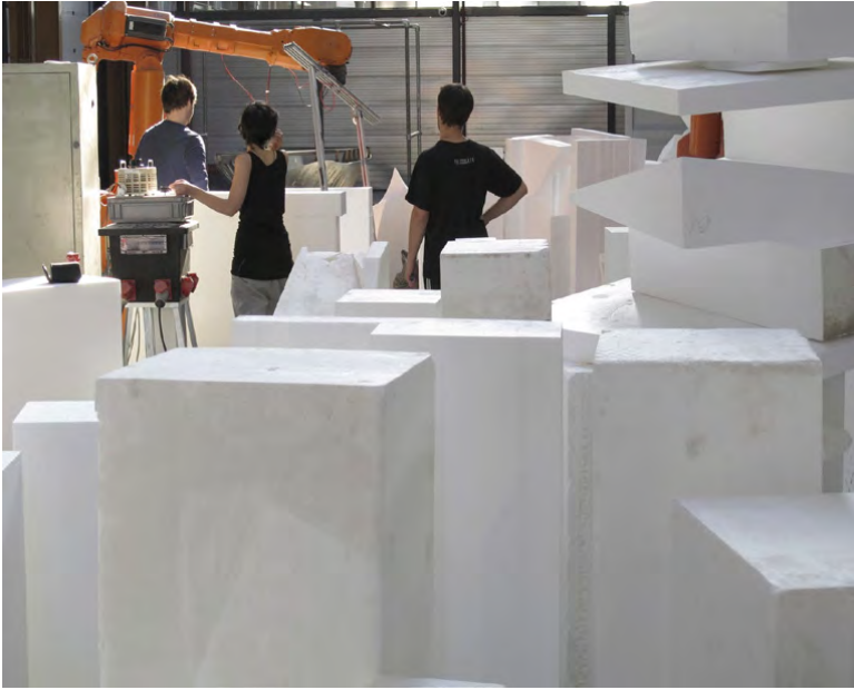
Figure 3.20: Ongoing production of the OptiCut formwork
