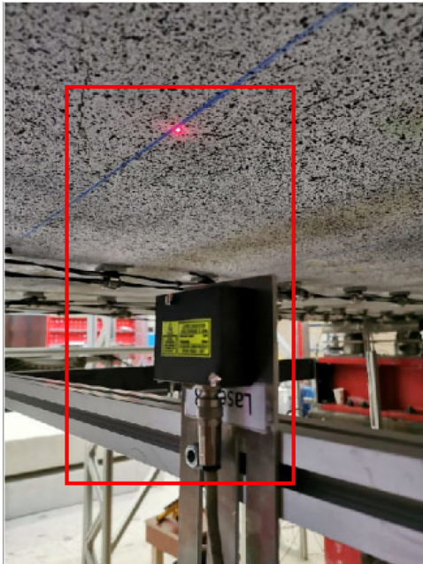
Figure 4. Application of laser distance sensor to measure the deflection.
