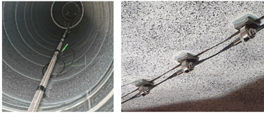
Figure 19. Application of FBG sensors. Left: glued to steel rebar, and right: attached to a concrete surface.
