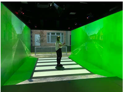
Fig. 1: Simulating road crossing behavior guided by the designed AR interfaces in the Highy Immersive Kinematic Experimental Research (HIKER) pedestrian lab at the University of Leeds.
