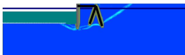
Fig. 11 Failure plane at critical acceleration as computed with PLAXIS 2D
