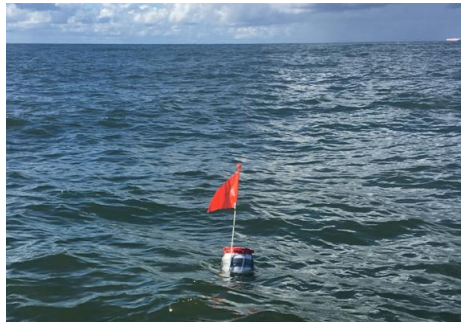
Figure 2.13: GPS-equipped surface current drifter deployed in the Ameland Inlet.
