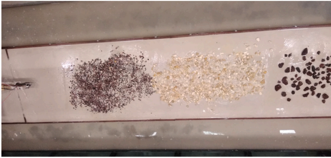
Fig. 15. The testing track filled with 15 cm sand into which nodules are half buried.
