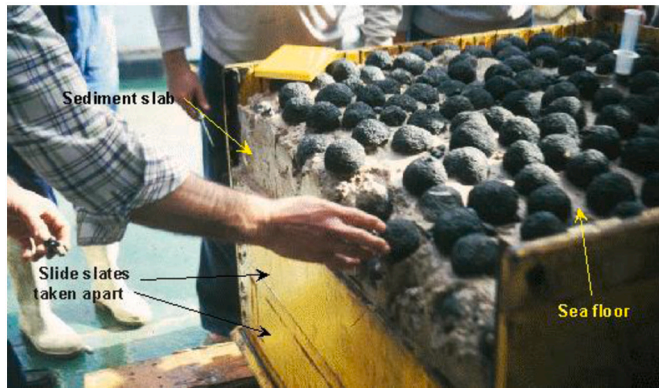
Fig. 1. Undisturbed nodule-sediment sample illustrating the burial of nodules (Museum National d'Histoire Naturelle Box Corer [19]).
