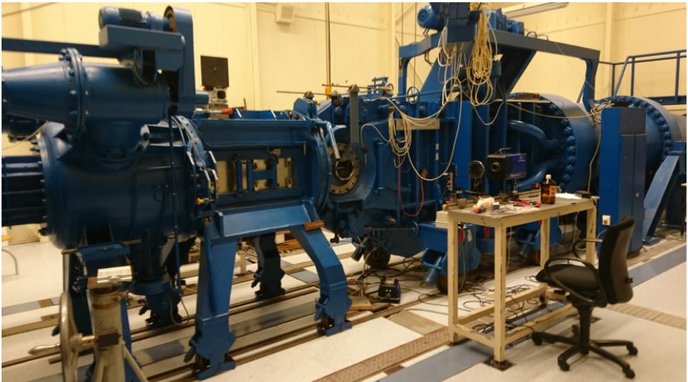
Figure 3.1: TST-27 Wind Tunnel (airflow from right to left).
