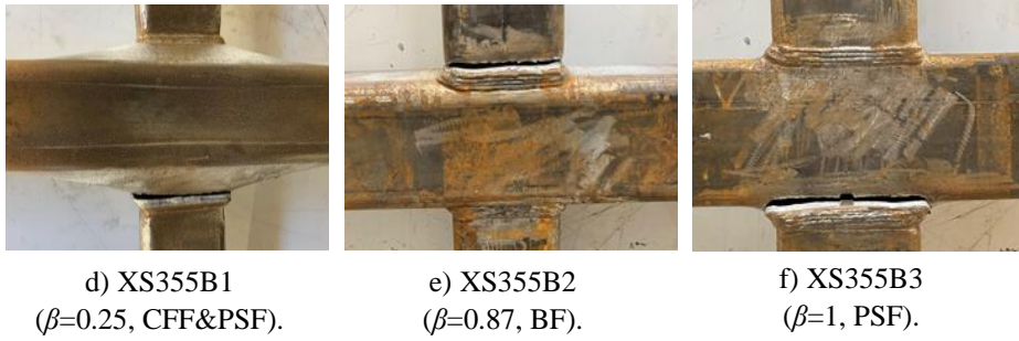
Fig. 6.7 Failure modes of S355 X-joints.
