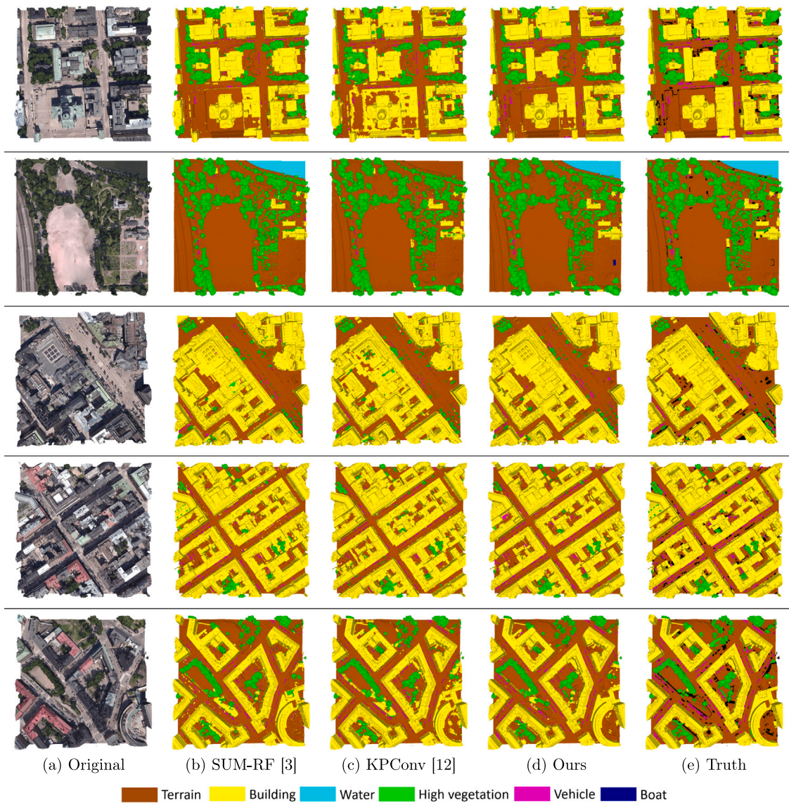
Fig. 13. Semantic segmentation results of SUM-RF (Gao et al., 2021), KPConv (Thomas et al., 2019), and our method on five tiles from the SUM dataset (Gao et al., 2021).
