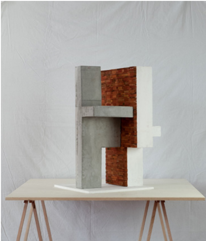
Fig. 11.1 Concrete and MDF model of the meeting of two walls from different times, scale 1:5, by Riccardo Garrone and Sam Stalker. Photograph: Bas Leemans.
