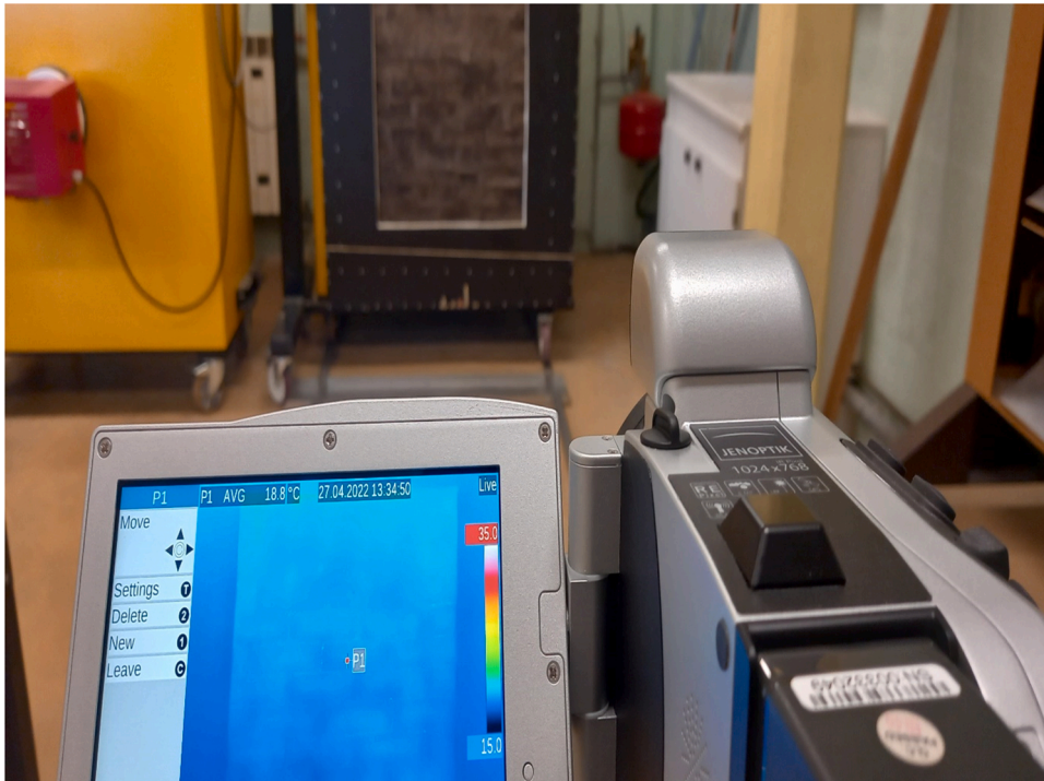
Fig. 16. Thermal imaging recording of S/BP wall surface exposed to ambient temperature.
