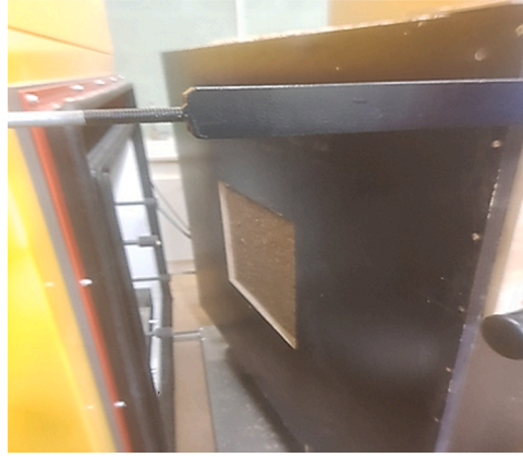
Fig. 12. S/BP wall insertion in the Thermo 3 device.
