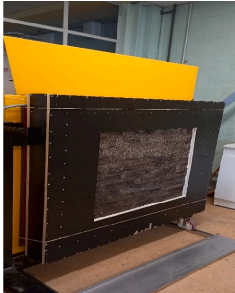
Fig. 15. S/BP wall fixed from one side to the hot climatic chamber and exposed to ambient temperature from the other side.
