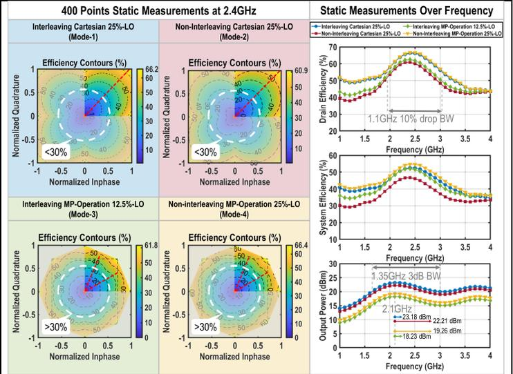
Fig. 4. Measured static DE contours of the first I/Q quadrant (left) and frequency responses, DE, SE, P<sub>out</sub>, (right) for different operational modes.
