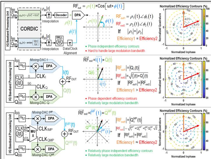
Fig. 1. Polar, Cartesian, and Multi-phase DTX architectures. Their operational concepts and corresponding efficiency counters' phase dependency comparison.
