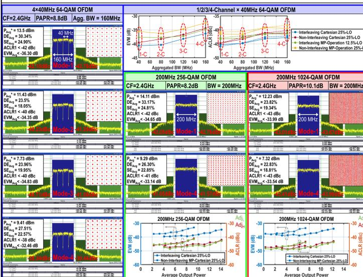
Fig. 5. Measured 4-carrier 160MHz 64-QAM OFDM (blue frame), single-carrier 200MHz 256/1024-QAM OFDM (green/red frames).
