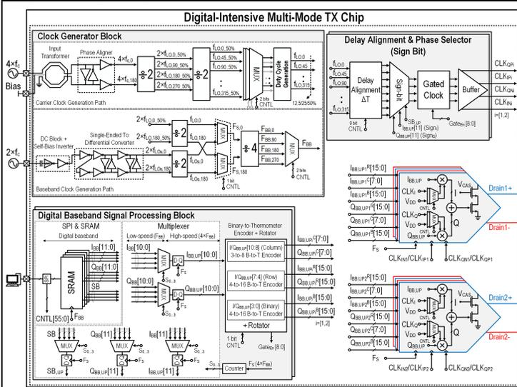
Fig. 3. The detailed block diagram of the proposed digital multi-mode transmitter.
