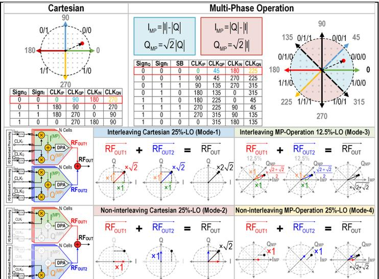
Fig. 2. The phase selectors of Cartesian and Multi-phase operation (top) and different (Non-)interleaving operating modes (bottom).
